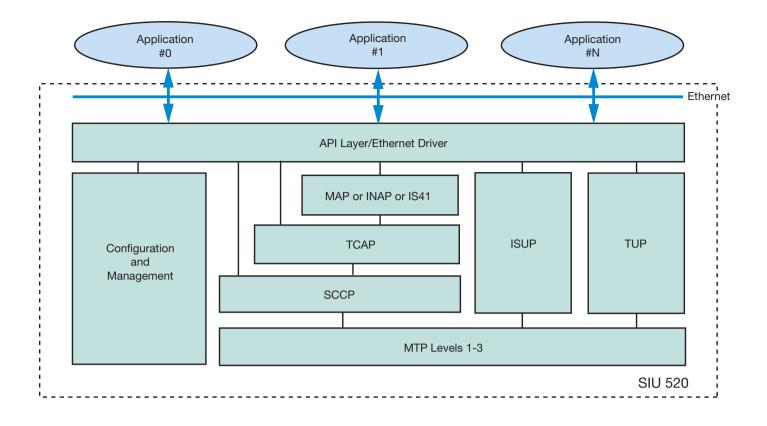
Figure 1. Structure of the Intel® NetStructure™ SIU520 SS7 Signaling Gateway
